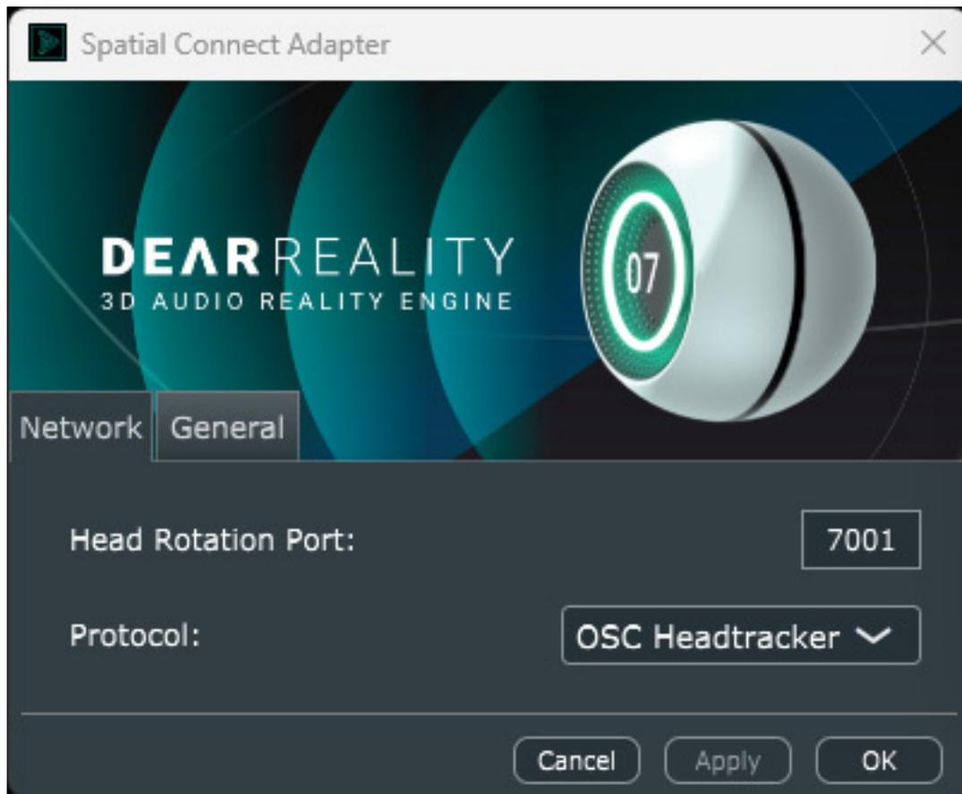
dearVR Monitor 2 from Dear Reality also supports head trackers. In the Bridgehead software, you have to select "dearVR" in the OSC dialogue. In addition to the Bridgehead software, installation of the Dear Reality software component "Spatial Connect Adapter" is required for connection (see illustration). "OSC Headtracker" is selected as the protocol here.
