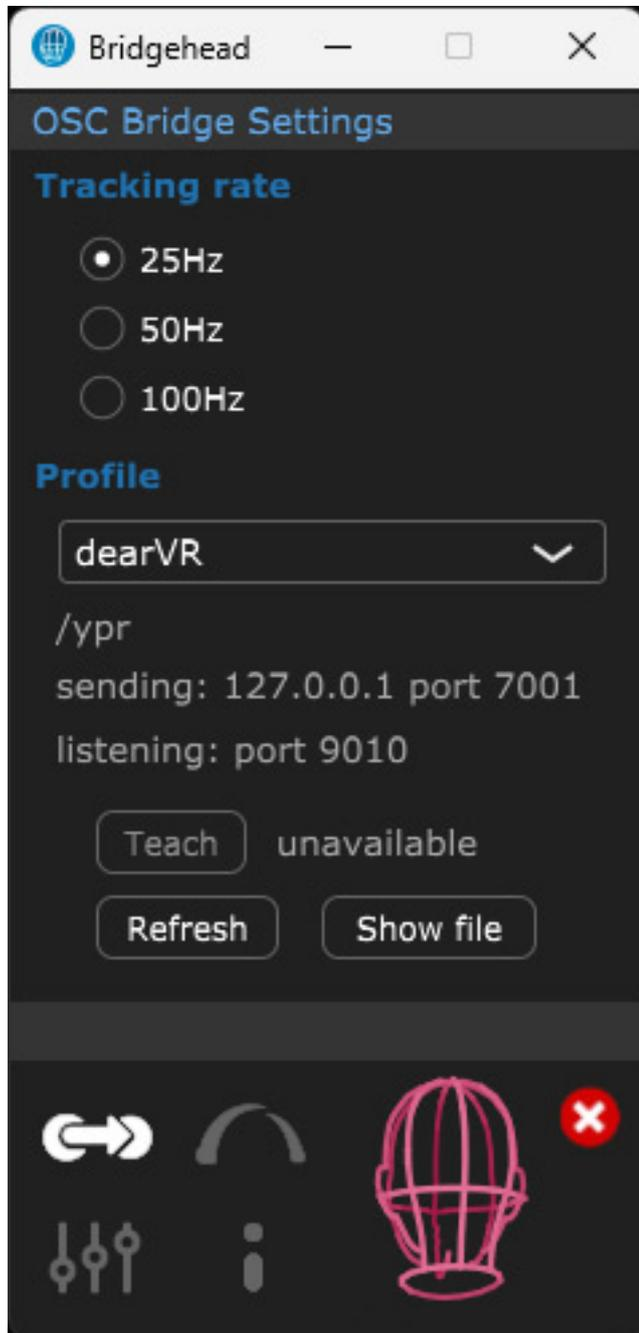
Communication between the head tracker and binauralizer plug-in takes place via the bridgehead using the OSC protocol. The position update data rate can also be set. In our experience, 25Hz is sufficient, and higher update rates may be too much for some DAWs.
