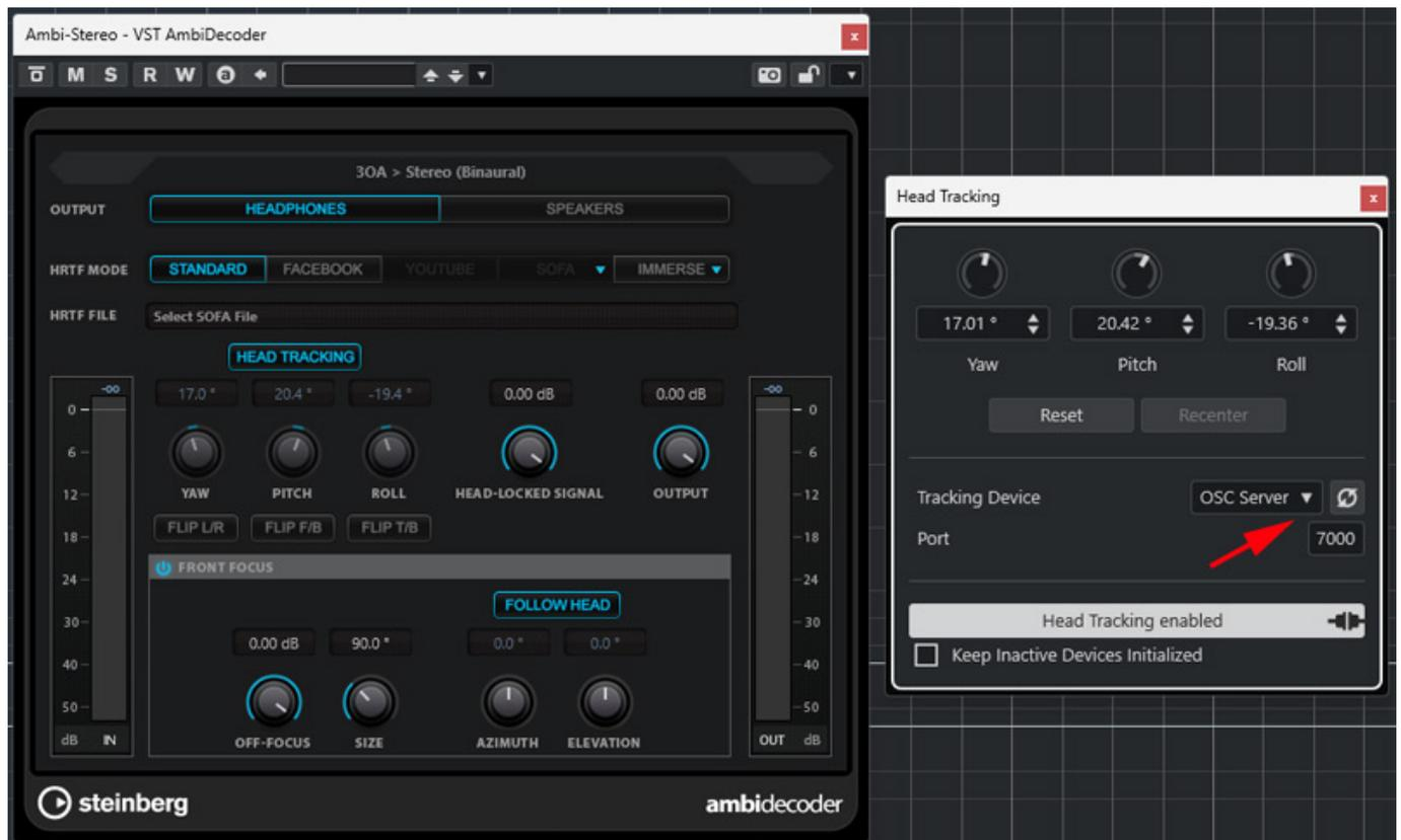
Then, you have to configure Cubase or Nuendo accordingly and activate head tracking in AmbiDecoder. We have already tested the AmbiDecoder. A look at the test can help with the configuration. Prior to this, head tracking must also be set to "OSC Server" and port 7000 in the corresponding Cubase/Nuendo dialogue (see illustration above). The dialog can be called from the Studio menu.
