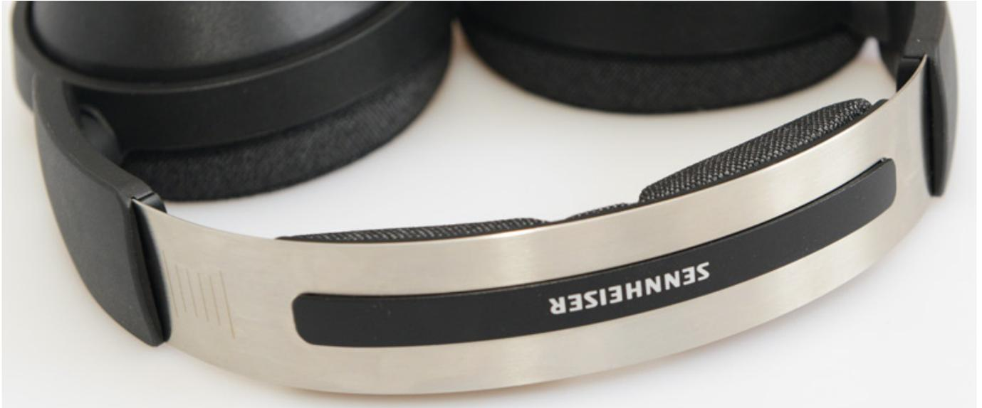
The Sennheiser HD 490 PRO uses a steel band as the headband. A plastic piece is attached over it. The width of this is very well suited for holding the head tracker band, and there is a small distance to the magnetisable metal band.
