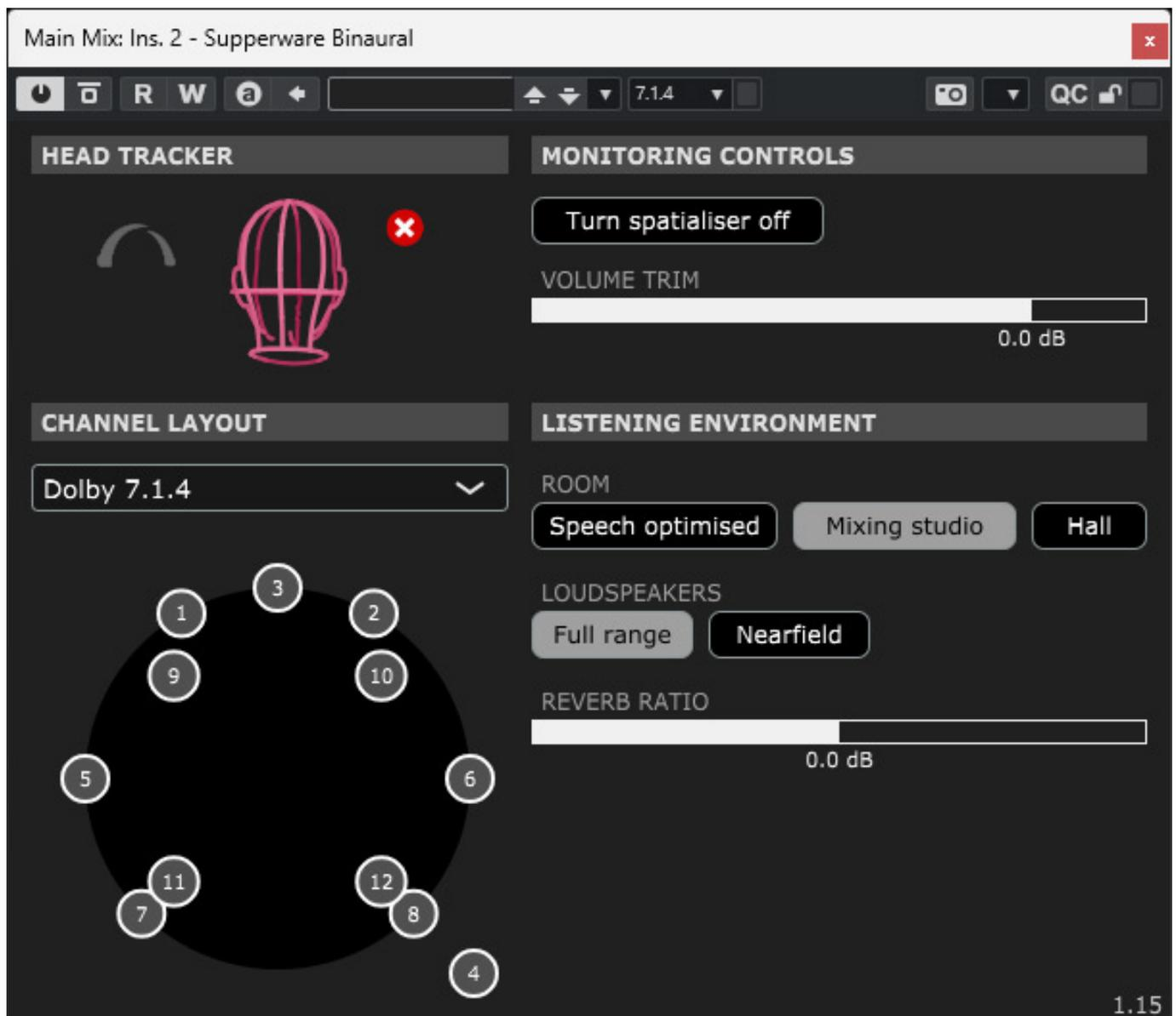
The plug-in provides binauralisation of input signals in speaker formats up to 9.1.6 and 22.2. It also offers room simulation with three selectable rooms (speech optimisation, mixing studio and hall) with adjustable reverb and selectable loudspeaker simulations (full-range or near-field monitoring).
