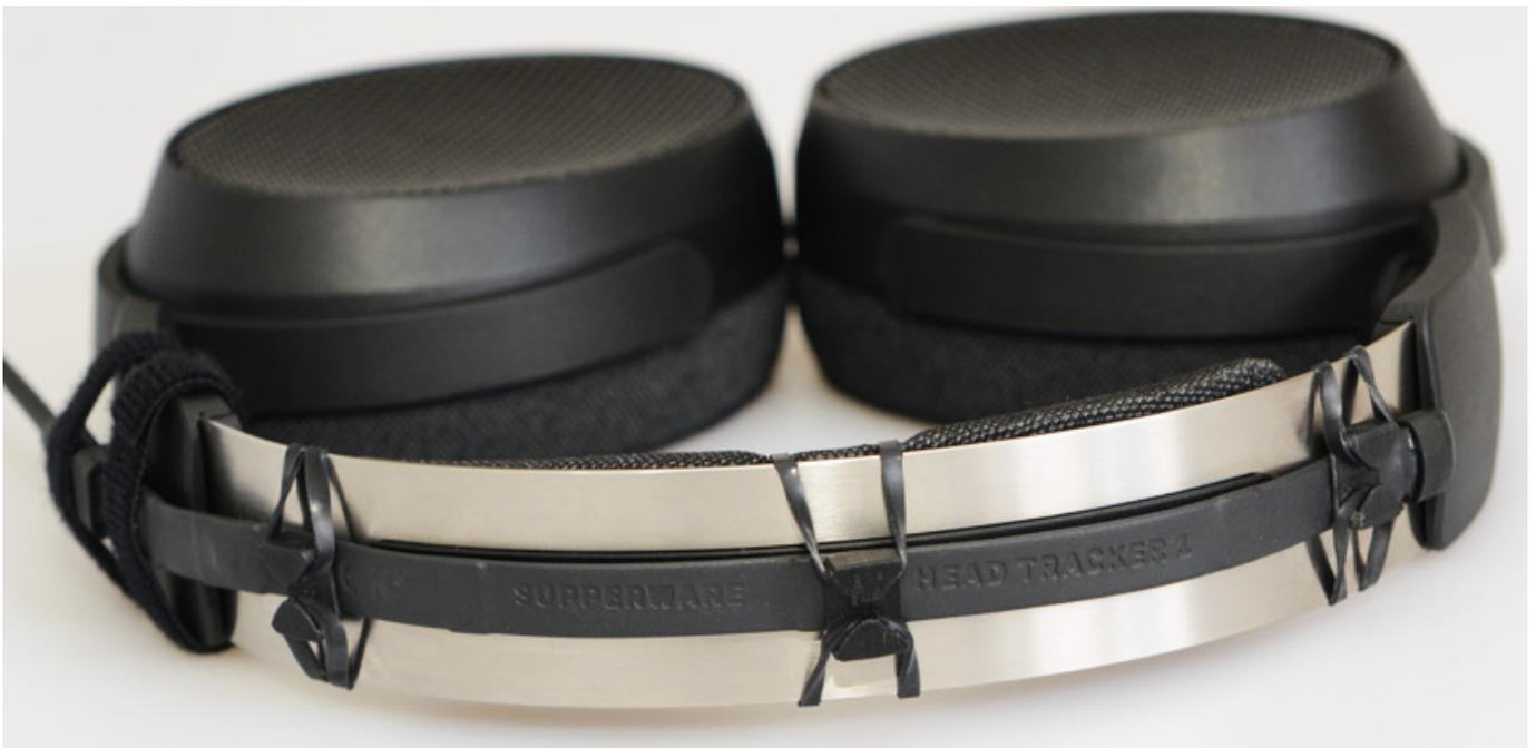
Using the Sennheiser HD 490 PRO as an example, we have shown how the head tracker band and USB cable can be attached using the rubber bands and clips provided and the two Velcro straps.
