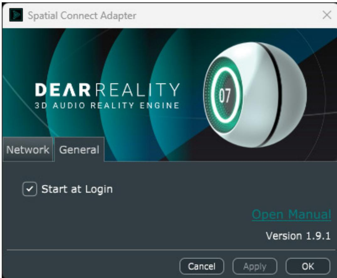
If you work a lot with the Headtracker and dearVR Monitor 2, it is recommended that this component is started automatically when the computer is booted (Start at Login).
