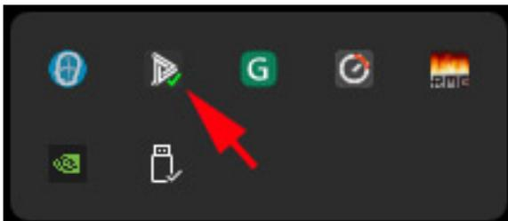
An icon is visible in the system tray after startup (see figure above), which is marked with a green symbol if connected to the head tracker (red if not connected).
