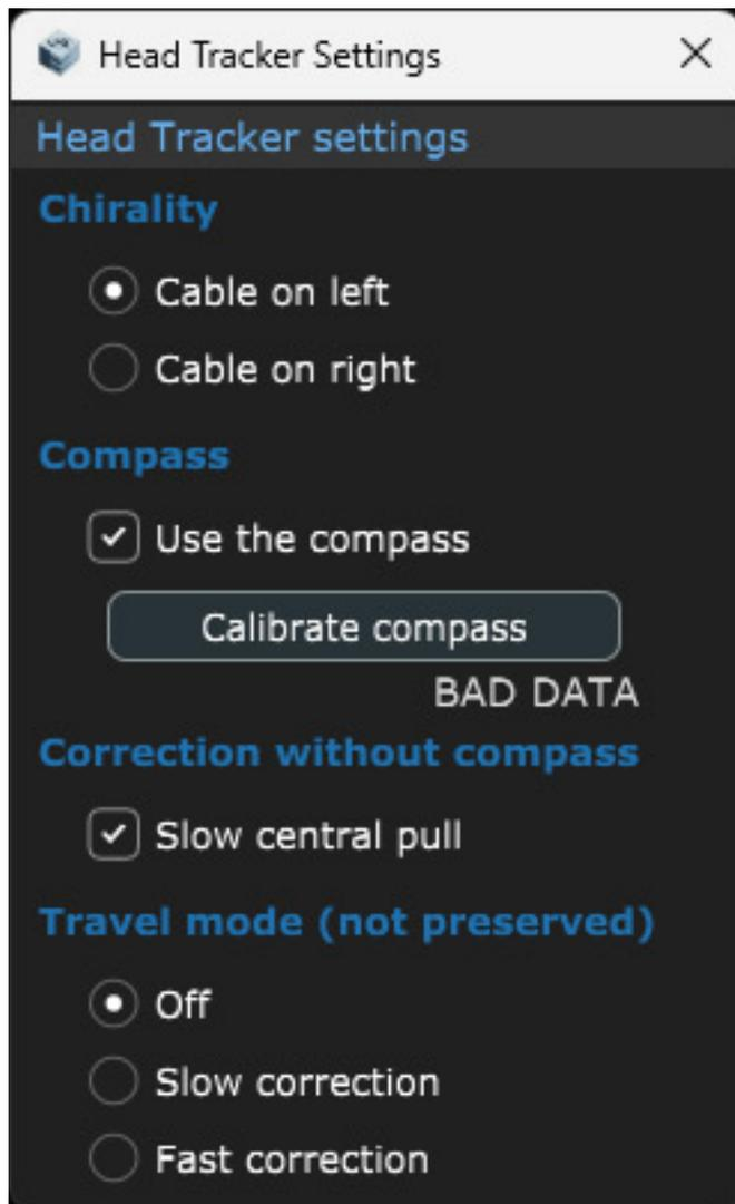
Basic settings and compass calibration are also possible. If the data is not being received correctly by the head tracker, this is also signalled (via the "BAD DATA" display, see illustration above). The advantage of the Supperware binauralization plug-in is that the Head Tracker 1 is natively supported, and no other software is required - only for calibrating the gyros/accelerometers or for firmware updates, if necessary.
