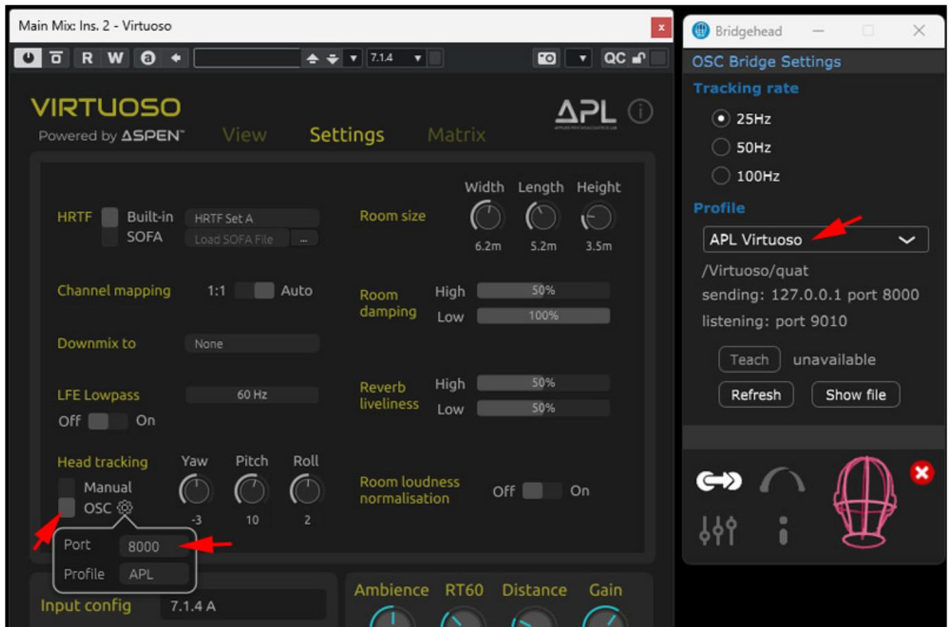
Connecting the Virtuoso binauraliser plug-in from APL is relatively simple. Select "APL Virtuoso" as the profile for Bridgehead, then activate head tracking via OSC in the plug-in, and adjust the port to 8000 if necessary.
