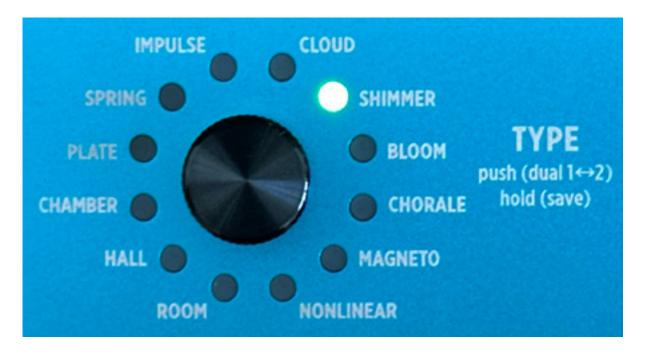
Let's go through the algorithms in detail. The IMPUSE algorithm is a brand-new algorithm that offers a convolution reverb with 22 selectable internal impulse responses of up to ten seconds in length. It is also possible to load your own impulse responses. I will discuss this more later.
