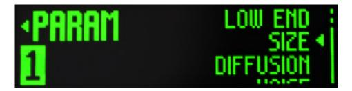
Briefly pressing the rotary encoder to the right of the display takes you to the menu with the individual preset parameters (see illustration above).
