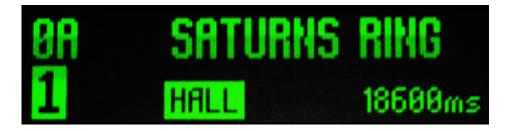
The normal display (see illustration above) shows the bank number and position (A/B), as well as the name of the preset. The first 50 banks are equipped with factory presets, and there are a 100 more banks for user-created presets. The display also shows which reverb engines are active, how they are connected, and the decay parameter value.
