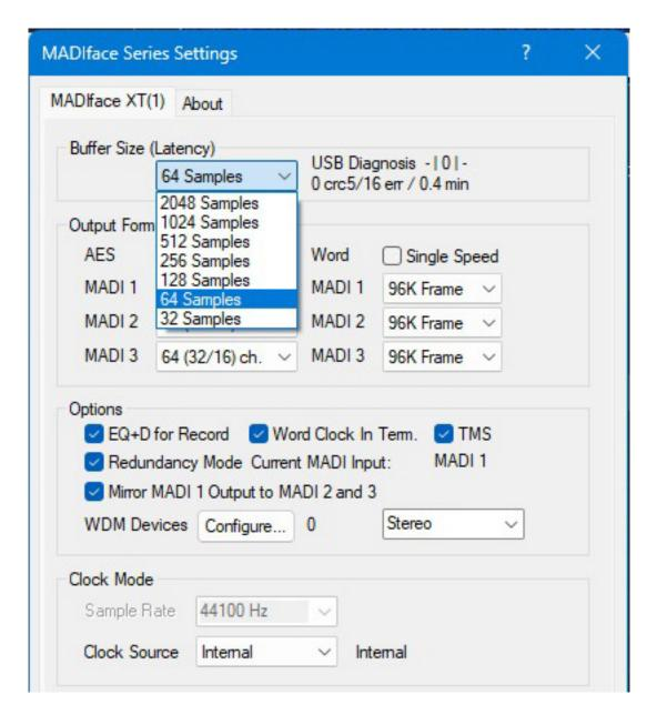
The flexible settings allowed extensive customization of the setup. Variable buffersizes from 32 to 2048 samples and latencies at a 44.1 kHz sampling rate with just 1.633 milliseconds input and 2.653 milliseconds output under Windows 11 were impressive and underline the professional standard that RME consistently pursues.
