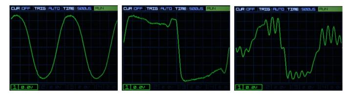
The DOOM switch has three positions: OFF, SUB, and BLOWN. In the OFF position, the function is switched off (Fig. left), in the SUB position (Fig. center), a signal with an octave lower is added, and in the BLOWN position (Fig. right), the level of the added signal is greater than the SUB setting, and there is a kind of decay, as you would expect from a speaker driven by a pulse (see figure above), but, as you can see, with very high-frequency components.
