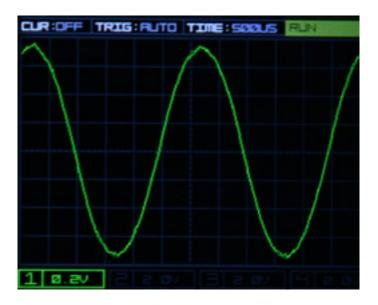
Let's take a look at how the individual parameters of the Dystorpia work. To do this, we apply a sine signal to the pedal input and observe on an oscilloscope how the output waveform changes when the knobs are moved.
