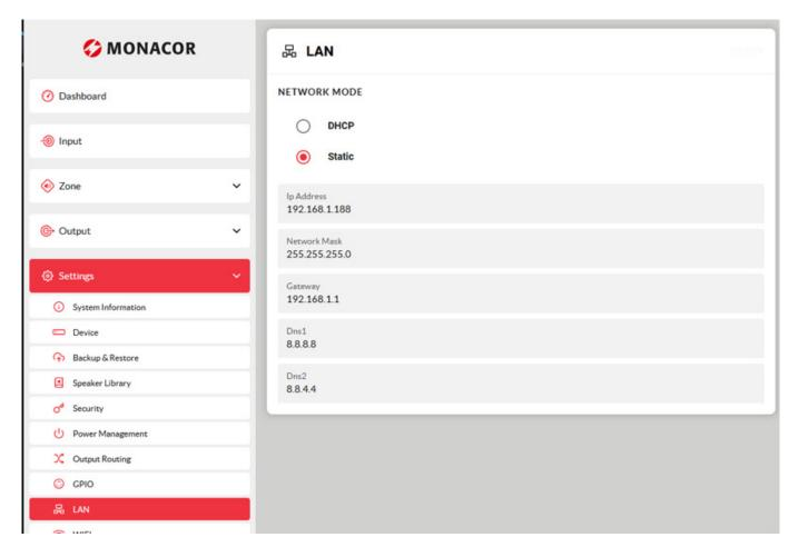
The IP address can either be set statically or assigned automatically via DHCP.
