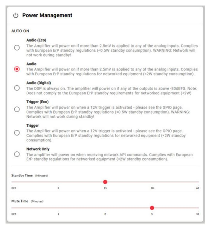
Extensive settings relating to power management can be made via selecting an operating mode as well as times for standby and audio mute (see image above). By the way, the power consumption in standby mode is under half a watt.
