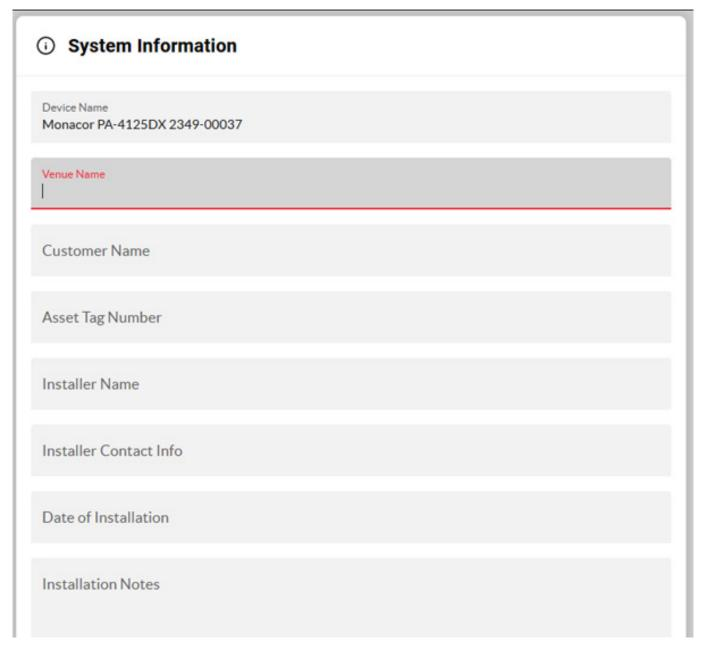
The user can enter the basic data for the amplifier via 'Settings'. The product name with serial number are default settings.
