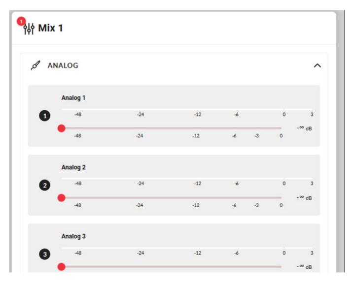
The PA-4125DX features 4 integrated mixers, each with 4 analogue inputs and SPIDF inputs as input sources. The names of the input sources and mixers can also be user-defined, i.e. click the mouse onto the name and select a different one, if required. However, the mixer does not feature a virtual mute button for the inputs. Instead, you have to move the fader all the way down.
