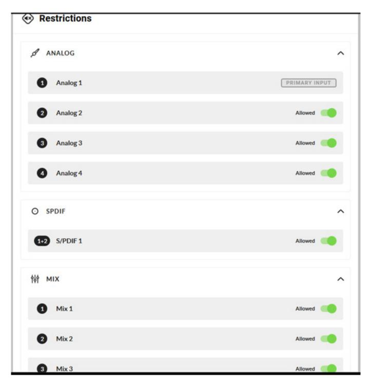
The dialogue 'Restriction' can be used to activate or deactivate individual inputs and mixers for the respectively selected zone (see image above).
