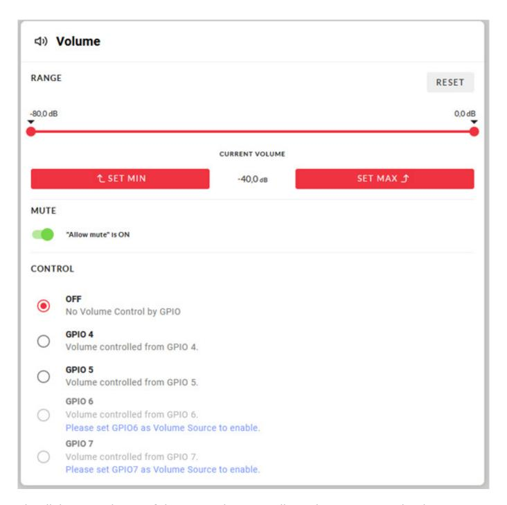
The dialogue 'Volume' of the respective zone allows the user to restrict the adjustable level range.
