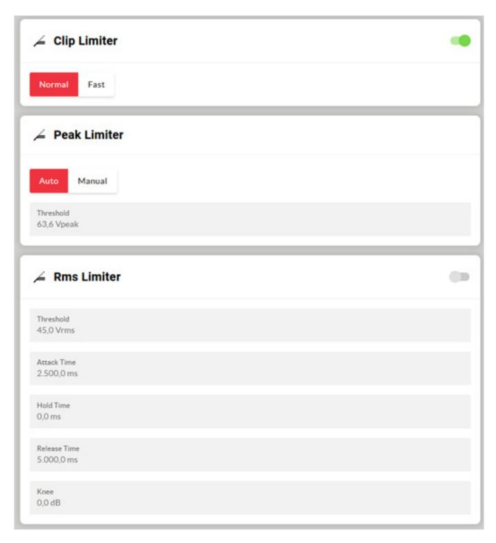
Furthermore, versatile things can be adjusted as presets, e.g. crossover frequencies, equalizer (also a 5-band equalizer), import of FIR filter coefficients and various limiters (see image above).
