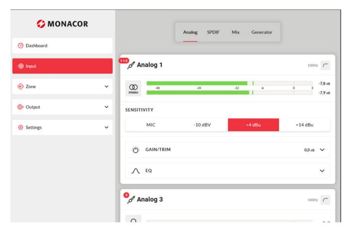
The sensitivity range of each analogue input can individually be adjusted via 4 virtual switches including microphone sensitivity and nominal line level +14dBu.
