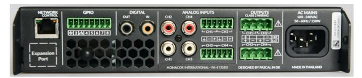
The PA-4125DX is equipped with 4 amplifiers. It can be operated in LoZ mode for connection of speakers with an impedance of 4 or 8 Ohms or using HiZ mode for 70V or 100V operation. However, this is only possible with 2 instead of 4 output channels. In LoZ mode, each amplifier features an output power rating of 125W and 250W for 70/100V operation.
