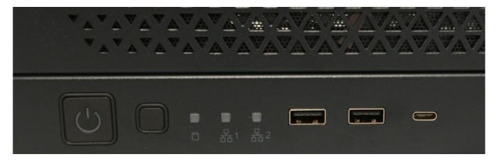
There are only a few operating elements on the front panel. In addition to the on/off button, there is a reset button and status indicators for hard drive activities and networks. There are also two USB-A ports (USB 3.0 with 5 GBit/s) and one USB-C port (USB 3, 5 GBit/s) on the front panel.
