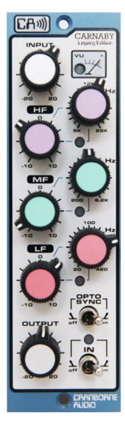
The input and output knobs are used for gain staging and offer 20 dB of level increase or decrease, respectively. An LED monitors the output level. The cutoff or center frequencies of the three bands can now be selected using the knobs arranged in pairs, and their levels can be adjusted by  $\pm$ 10 dB in 0.5 dB steps.
