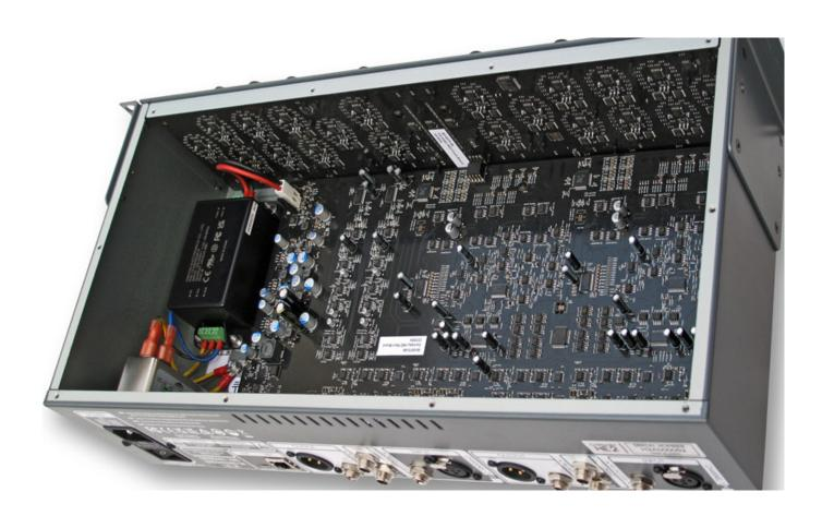
Anyone who assumes that the Carnaby HE2 simply contains two boards of the 500 module plus some peripherals is far from the truth: the HE2 has completely redesigned boards with high-quality electronics. According to the manufacturer, the proposed solution enables better audio performance and simpler integration of digital controls. In addition, manufacturing costs are reduced when a single board is used.
