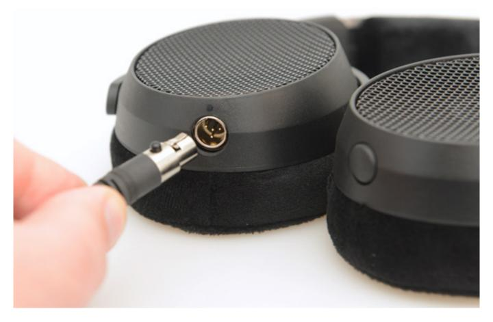
Another pleasing feature is that the headphones have mini XLR sockets in both ear cups. This means that you can use the connection on the right or left and cover the connection that is not in use with a rubber plug.
