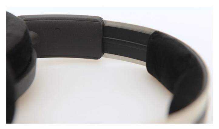
The headband can be moved by approx. 37 millimetres on each side, i.e. approx. 75 mm in total. The headband extension is notched, and there is also a scale on the top so that the extension can be adjusted equally on both sides.
