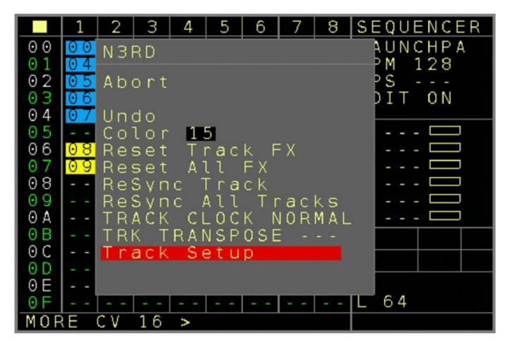
The CV16 module also offers eight ASR envelopes. These can be set via the NERD menu and the TRACK SETUP menu item when the corresponding track is selected.
