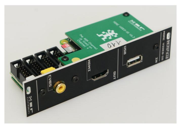
The video module is a relatively new and offers a wide range of functions. It is connected to the NSA and MIDI bus. However, it is still possible to operate a MIDI expander as usual. The video expander appears in the system as NSA slot 4. The module must also be connected to the MIDI bus. The cables for the connection are, of course, included in the module.
