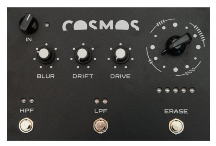
The three knobs on the left side of the COSMOS display different functions depending on the algorithm, or sometimes no function at all. The DRIVE knob can be used to achieve targeted saturation or overdrive, where the signal is slightly compressed and distorted. However, this knob also has a different function for certain firmware variants.
