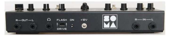
A USB 2.0 socket can be used to connect a FAT32-formatted USB stick to load the firmware. This does not necessarily require an update, but rather there are different firmware versions for different application scenarios. If a firmware file is located in the root directory of the inserted USB stick, will be loaded by pressing the RECORD button and the turning on the device.
