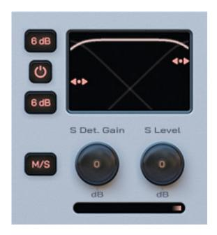
Below these controls, knobs that provide different parameters depending on the input configuration are available. This allows the LFE level(s) to be adjusted. gravitas can also handle multiple LFE channels. In stereo mode, an M/S section appears here instead of the LFE knob (see illustration above). MS processing can also be deactivated, and the side detector and side levels can be changed.
