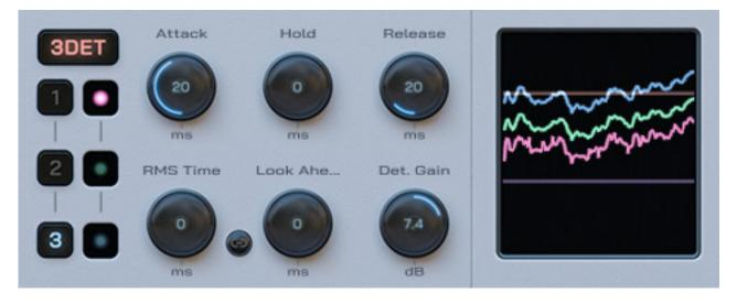
The 3DET button can also be used to activate three parallel detector settings instead of one, whose detector input gain can then be adjusted using the "Det. Gain" knob. The knobs, or symbolized values, are then reddish, greenish or bluish depending on the selected detector, and the three detector level curves are then also shown in the display, as well as the two threshold values set in the signal path.
