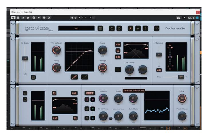
Depending on the host software and plug-in, up to 128 channels can be processed, for example, in Reaper. With Nuendo as a VST3 plug-in, the maximum number of channels is 64. Another feature worth mentioning is the use of the module in Fiedler Audio's Dolby Atmos Composer. This means that up to 128 channels of an entire Dolby Atmos mix can be edited using gravitas MDS.
