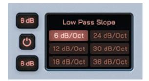
To the right of this, a filter (high/low pass) can be setup and, if necessary, deactivated. The cut-off frequencies of the two filters can be set using the mouse. Clicking on one of the two labels below and above the on/off switch opens a dialog for selecting the filter slope between 6 and 36dB/oct. in 6dB steps.
