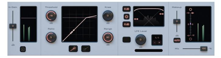
The next section displays the signal processing path. Here, you will find virtual level meters at the input and output as well as knobs for the input gain (In Gain) and output gain (Makup), which can also be switched to automatic adjustment using the
