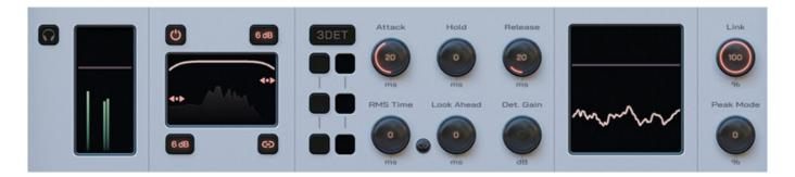
The lower section deals with the detector level and the control variables. There is also a high-pass/low-pass filter in the detector path, which can be set as described in the audio signal path above. The filter settings for the signal and detector path can be linked via the icon on the right below the filter graphic.
