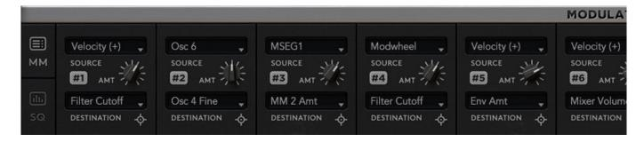
The modulation matrix can be operated in the lower section. Here, twelve modulation sources can be switched to modulation destinations, and the modulation index can be varied. The DESTINATION icon can also be used to link modulation destinations with the mouse.
