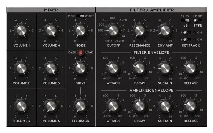
The mixer was thus upgraded with six controls for the oscillators and the noise generator (white/pink noise). There is a drive control to deliberately provoke saturation behaviour and a feedback control that feeds the output back to the input via an attenuator.
