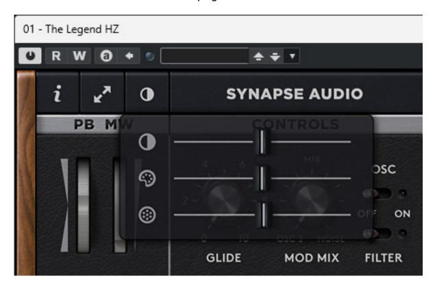
The size can be set in steps via a menu or continuously with the mouse. Global brightness, virtual LED intensity, and background can be adjusted using controls (see illustration above).
