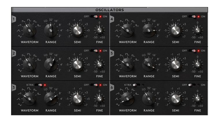
We now arrive at a significant difference from the original design. On the left, everything still looks original; however, instead of three, The Legend HZ version now fortunately has six oscillators. Therefore, oscillators 1 to 3 are functionally present twice. Keyboard tracking can be switched off for oscillators 3 and 6. Compared to the original, "Sharktooth" has been added to the waveforms - a mixture of sawtooth for the rising, and a triangle waveform for the falling waveform.
