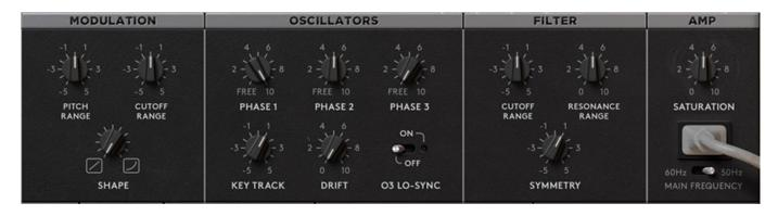
Under MODULATION, the user can limit the modulation wheel range, adjust the effect of the wheel on the filter frequency, and switch continuously between linear and exponential response of the wheel. The linearity of the keyboard tracking can also be shifted to higher or lower frequencies. With DRIFT, you also have an adjustable random size, and with the "Oscillator 3 Low-Sync" switch you can synchronise it with the DAW host tempo.
