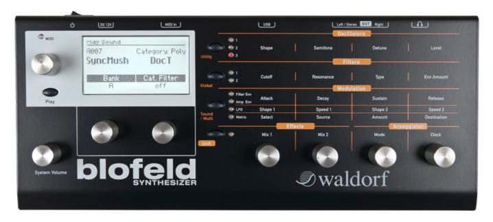
Many Waldorf synthesizers are based on the concept of the PPG synthesizers, such as the Waldorf Q, Micro Q, and Microwave, i.e., several wavetable-synthesis-based oscillators followed by filters and VCAs. The same applies to the Blofeld. The design uses three digital oscillators. However, instead of analog filters and VCAs, virtual ones realized via DSP are used. This makes it possible to use up to 25 voices.
