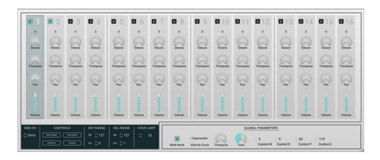
The Multi Mode can be activated via the MULTI page, where up to 16 so-called Multi Parts can be activated and set. The parameters that can be set here are Detune, Transpose, Panorama and Volume per Part. In the lower area, global settings can be made for all 16 parts. The parts can be overlaid or split.
