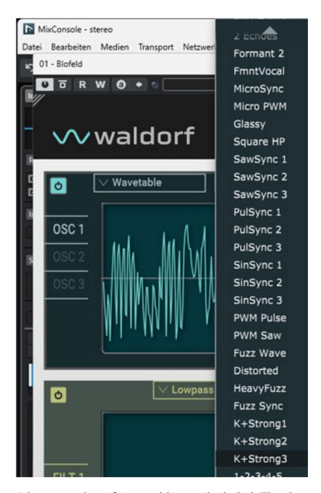
A large number of wavetables are included. The three wavetables labeled K+Strong 1 to 3 have a special status. These are not stored wavetables but three Karplus-Strong string synthesis algorithms that are calculated in real time.
