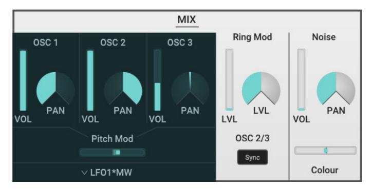
Each oscillator can be adjusted in level and stereo panorama in the MIX block. A ring modulator can also be used here and there is also a noise generator with adjustable coloration.
