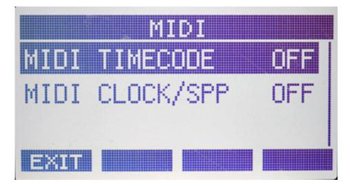
MIDI Timecode (MTC) and MIDI Clock with SPP (Song Position Pointer) can be output via USB and MIDI during recording and playback. However, Studio Bridge cannot respond to incoming signals as a slave.
