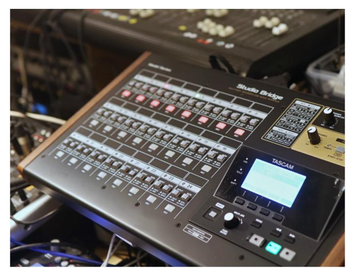
Studio Bridge is in the format of a desktop device. With a separately purchased kit, Studio Bridge can also be mounted in 19-inch racks. To do this, you have to remove the visually appealing side panels with a wooden finish. On a table or stand, the Studio Bridge stands at a slight angle. With dimensions of 446.5 x 114.6 x 269.5 mm, it weighs 4.5 kg.
