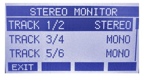
The routing of USB channels 1/2 at the mixing console can be changed.
