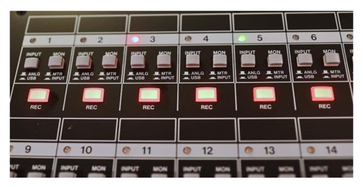
A push button switch can be used to set whether an analog or USB signal is to be applied to each input or channel. Another switch next to it allows you to switch between "MTR" and input. MTR stands for multitrack recorder. So you basically switch between a playback signal from the recorder and the input signal for all outputs. Below that is a recording button that you use to arm the track for recording. During recording, the button lights up red, and in standby mode, the button flashes.
