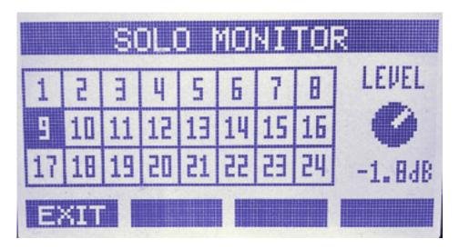
Clicking on the Solo entry will also take you quickly from the second main menu page back to the solo monitor display, where soloed tracks are marked in black. Adjacent tracks can be switched to stereo in the stereo monitor menu to listen to them in stereo. Alternatively, all tracks with a center stereo panorama setting end up in the mix as mono.
