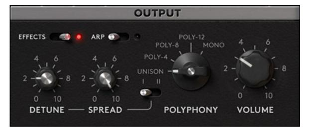
Various polyphony modes can be set in the OUTPUT section, ranging from MONO to UNISON (four voices are triggered simultaneously) to polyphony with four, eight, or
