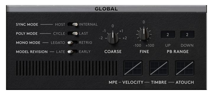
Here, you can set different sync/trigger modes and two different model revisions with slightly different oscillator and filter tolerances. There are also coarse and fine tuning, pitch bend range limits (up to +/- seven semitones), and three parameters for MIDI Polyphonic Expression mode, as The Legend HZ also supports MPE.
