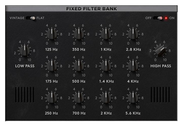
Yes, and then there is another delicacy from the 5 U Moog modular system: a virtual Moog 914 filter bank with twelve band-pass filters as well as a low-pass and a high-pass filter. The corresponding filter bands can be boosted or attenuated using the controls.
