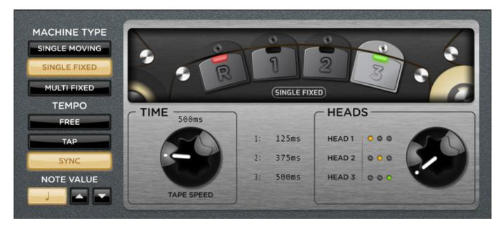
In SINGLE FIXED mode, one of the three fixed-position heads can be selected, and the tape speed can be continuously adjusted.
