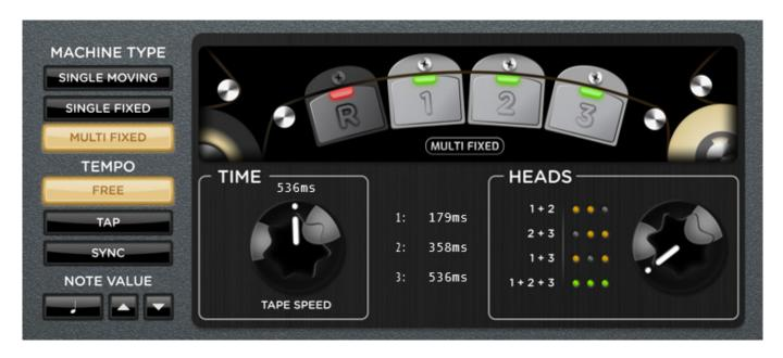
In MULTI FIXED mode, the three playback heads are also fixed, and the tape speed can be varied. Instead of one, two, or all three heads can be activated. The TEMPO can be freely selected or synchronized with the DAW tempo and then based on note values. It is also possible to enter this using TAP.
