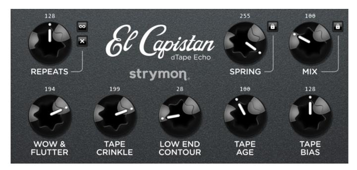
The number of repetitions, the temporal modulation via wow and flutter, and the transmitted effect bandwidth (TAPE AGE) can be set at the bottom. There is also a spring reverb effect, the strength of which can be adjusted using a knob (SPRING), and a mixing knob for the ratio of the original signal to the effect signal.
