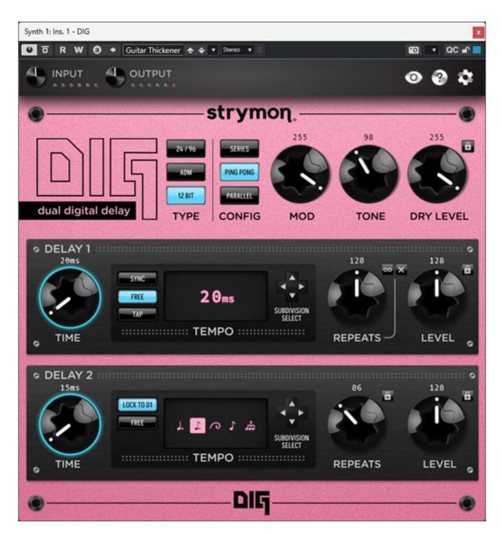
At the top, you can adjust the input and output levels. There is a bar graph for each, and three icons can be used to switch the parameter value output on and off to access help and global settings dialog. The plug-in is divided into three sections: one for the global parameters at the top, and one each for delay 1 and delay 2.
