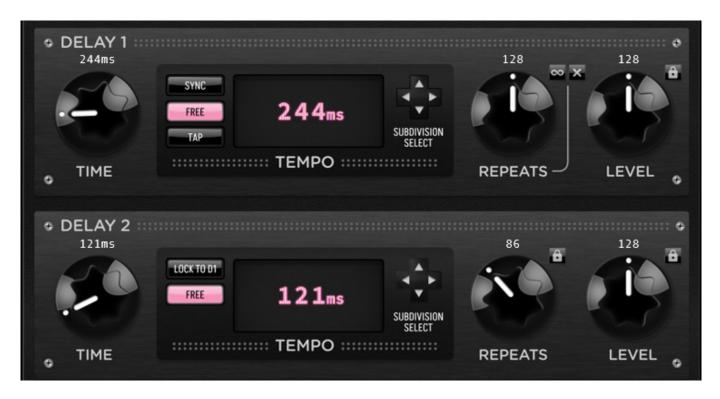
In the two lower sections, the delay time and echo repeat count can be set for each delay. The two delays can be operated independently or synchronized. The virtual button TAP allows you to set the tempo by clicking.
