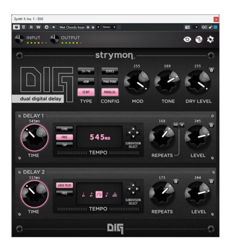
Let's start with the DIG Dual Digital Delay. As the pedal model is designed in pink, the GUI can be switched between pink and black. The user interface includes everything the hardware pedal offers (six encoders and four switches), but there are additional settings.
