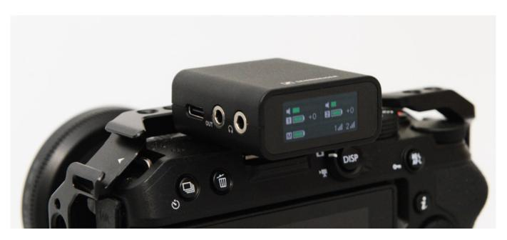
The supplied hot shoe adapter allows the camera to be used (here a Nikon Z30 as an example).
