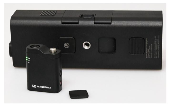
Now to the transmitter, which measures 42 x 33 x 21 mm. It weighs 27 grams and has a clip on the back for attaching it to clothing. However, there are also two magnetic plates in the multifunctional bar. The clip is also magnetic, transmitter can be easily attached to clothing without a collar, such as a T-shirt. The transmitter has an integrated omnidirectional condenser microphone. The maximum permissible sound pressure is 113 dB SPL (@ 1 kHz, 1 m).
