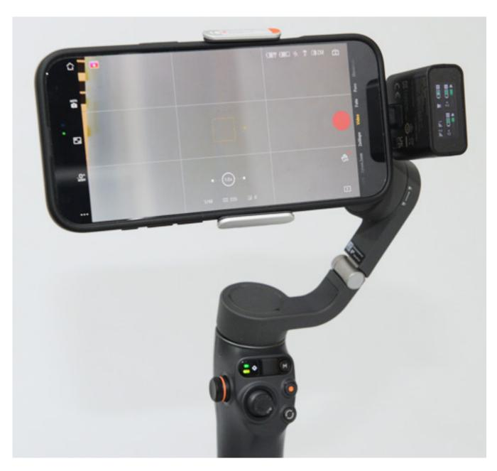
The transmitters are so light that you can easily mount them on a camera with a gimbal - you only have to slightly change the center of gravity if necessary. In connection with an iPhone Pro Max 16 and a DJI Osmo Mobile 6, the operation worked perfectly (see figure above).
