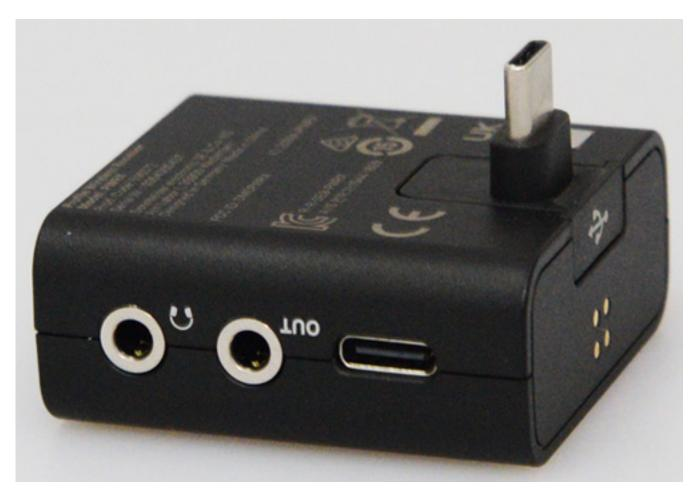
However, the two 90-degree adapters USB-C to USB-C (see figure above) and USB-C to Lightning plug are also interesting. This allows the receiver to be connected
