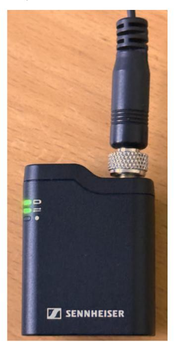
Thanks to the 3.5mm TRS jack, an external microphone can also be connected. The picture below shows how small the transmitter is compared to the jack plug.
