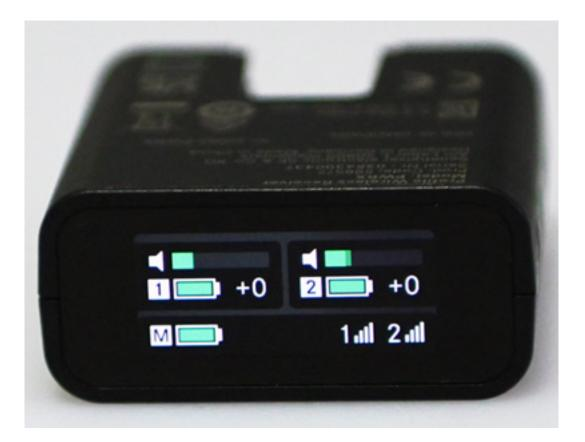
The receiver is also extremely compact and lightweight, measuring  $45 \times 42 \times 19$  mm and weighing only 30 grams. This device has an OLED display and a 350-mAh battery with an operating time of approx. seven hours and a full charging time of two hours. The profile wireless receiver also has an integrated headphone amplifier. Headphones with an impedance of at least 32 ohms can be connected here. The output power is 25 mW.
