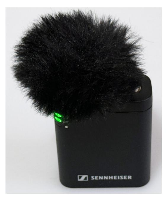
The supplied windscreen is placed on the microphone and locked by rotating it.
