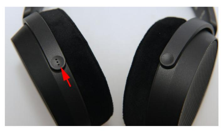
Tactile markings for headphone orientation on the HD 490 PRO are an excellent idea. For the correct wearing direction, there are two indentation marks at the back, and three dots (see illustration above) are embossed on the left-hand side of the headphone cup. When you hold the headphones in your hand, you can immediately feel whether they are correctly aligned.
