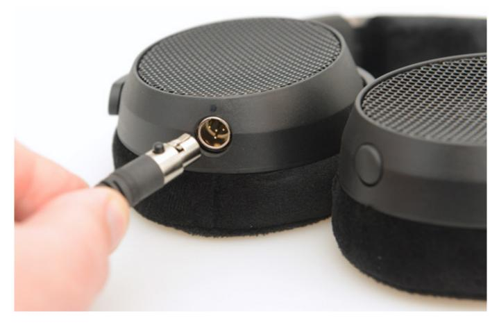
Another pleasing feature is that the headphones have mini XLR sockets in both ear cups. This means that you can use the connection on the right or left and cover the connection that is not in use with a rubber plug.
