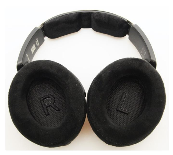
The two ear cups of the headphones can also be folded down so that the headphones can lie flat on the table. The channel designations are also clearly marked on the inside of the ear cups.
