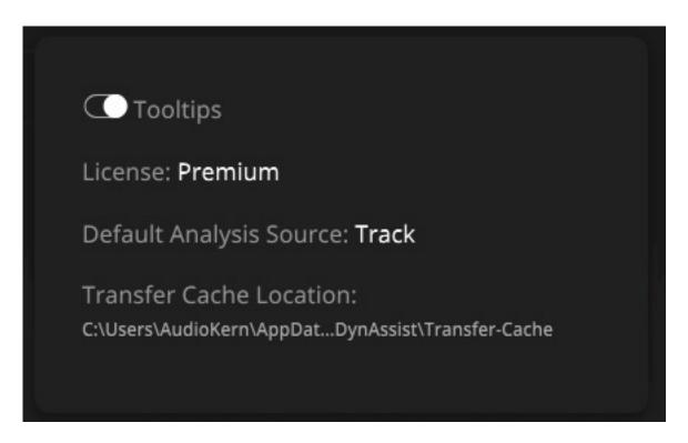
The global settings (accessed via the gear symbol) can then be used to select whether the general analysis source is a track or an event (see figure above) and tooltips on mouse-over can also be activated. Presets can also be saved and loaded in the top-left corner of the GUI. Some factory presets are also provided here.
