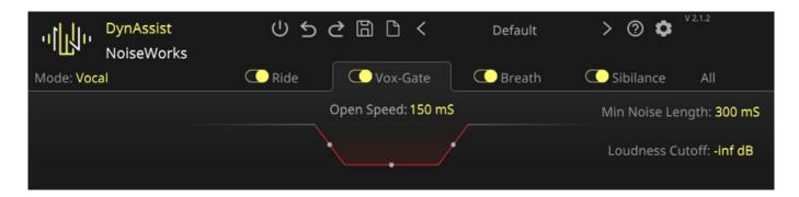
The gate's rise and fall times as well as the reduction can be set using the graphic. The "Min Noise Length" parameter allows the user to specify whether a region is detected as noise or a speech pause. Then, there is the "Loudness Cutoff" parameter in Vocal Mode, which sets an additional threshold for voice activity, while the gate's threshold can be set in Instrument Mode.
