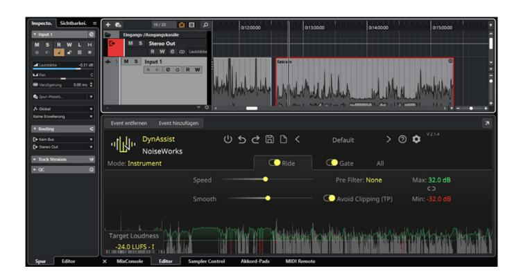
After double-clicking on the corresponding event, a corresponding editor opens below the tracks, in our case the DynAssist user interface (see figure above).
