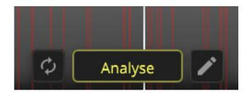
With two buttons, you can automatically analyze each time a parameter is changed or to manually analyze a specific selected area. The latter makes sense, for example, if you want to change several parameters without analysis in between. You can open the editor using the pencil symbol (see figure below).
