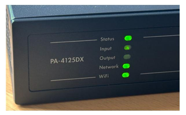
The device is operated completely via the built-in HTML5 web server. There is also an Ethernet connection on the rear panel for integrating it into a local network as well as a 2.4 GHz WLAN which operates as an access point or as a client. The device is delivered in access point mode. Initial configuration is done using a standard password.
