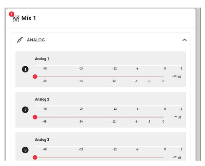
The PA-4125DX features 4 integrated mixers, each with 4 analogue inputs and SPIDF inputs as input sources. The names of the input sources and mixers can also be user-defined, i.e. click the mouse onto the name and select a different one, if required. However, the mixer does not feature a virtual mute button for the inputs. Instead, you have to move the fader all the way down.
