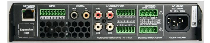
The PA-4125DX is equipped with 4 amplifiers. It can be operated in LoZ mode for connection of speakers with an impedance of 4 or 8 Ohms or using HiZ mode for 70V or 100V operation. However, this is only possible with 2 instead of 4 output channels. In LoZ mode, each amplifier features an output power rating of 125W and 250W for 70/100V operation.
