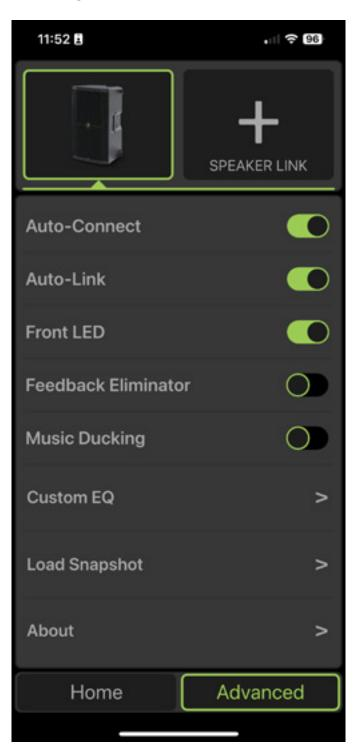
In "Advanced Mode", the app provides additional functions. For example, a custom equalizer for the main output. However, this only has a low-shelf and a high-shelf band.
