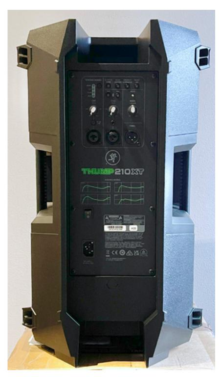
Both input channels and the main channel have separate gain or volume potentiometers. Channel 1 of the Thump210XT can be switched from line to
