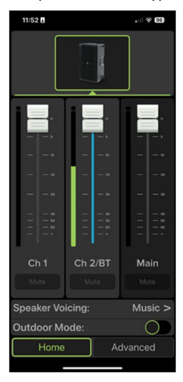
Apart from operating the system directly on the active module, the Mackie Thump210XT can also be controlled remotely via the free "Thump Connect 2" remote app. The app is available for both iOS and Android users to download. The connection with the app is also realized via Bluetooth and works simultaneously with the Bluetooth stream. The design of the Thump Connect app is basically self-explanatory. The home screen presents an overview of the incoming signals,
