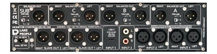
First of all, let's look at the outputs. There are three balanced (XLR jacks) stereo outputs and a switchable subwoofer output (mono, XLR jack). Furthermore, two stereo slave outputs (XLR jacks) are available, which are buffered but not regulated. All outputs offer a maximum level of +26 dBu and an output impedance of < 1  $\Omega$ . The headphone output on the front panel is available as a 3.5 mm stereo jack, as well as a 6.3 mm stereo jack.
