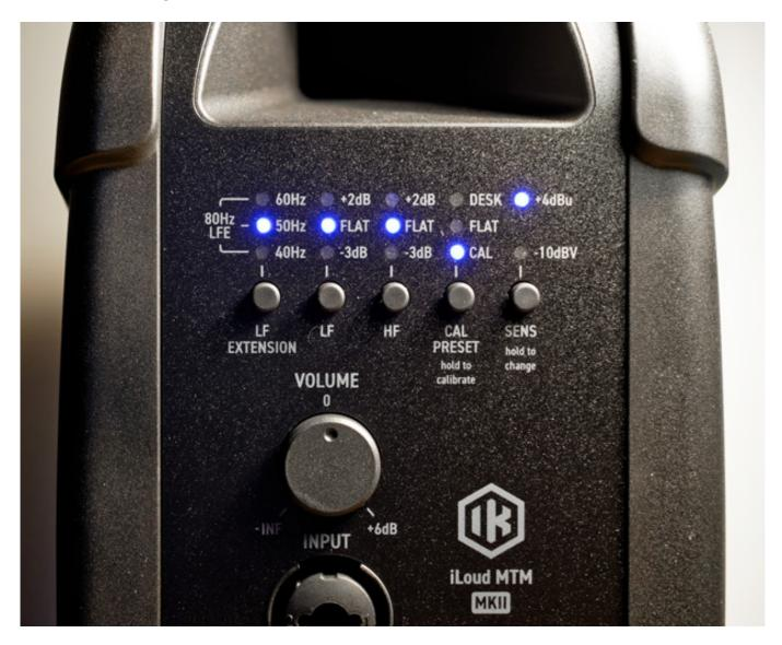
The models also feature a four-stage low-cut filter that acts as standard below 50 Hz but can also be set to 40, 60, or 80 Hz depending on the application and necessity. The last mode is designed for use with additional subwoofer units or bass management in conjunction with multichannel setups.
