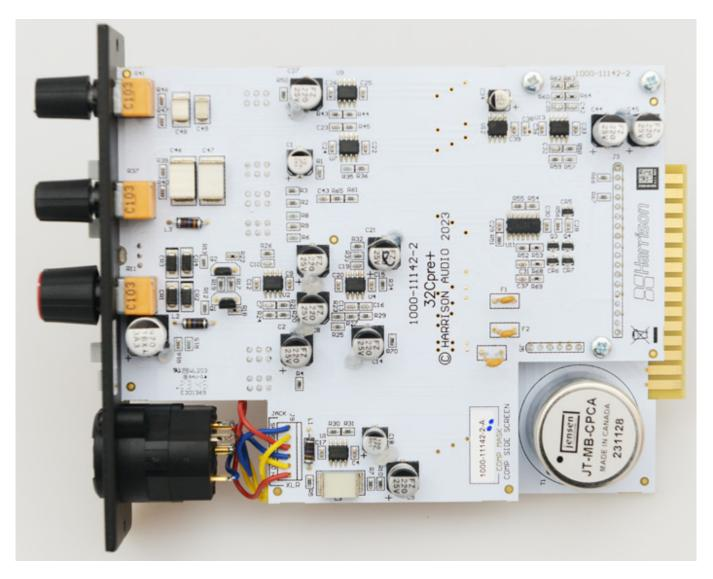
In line with the Harrison classic, a Jensen transformer is located in the signal path; in this case, a JT-MB-CPCA with first-class performance data. According to the manufacturer, the input gain of the module is between +20 and +70dB. This means that there is also enough power to operate vintage ribbon mics. A multi-coloured LED visualizes the input level very reliably.
