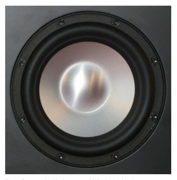
The woofer was updated in the summer of 2024. Previously, a Honeycomp cone was used that was coated with glass fiber on both sides. A multi-layer aluminum cone is now used, which is coated with plastic to tune resonances lower.
