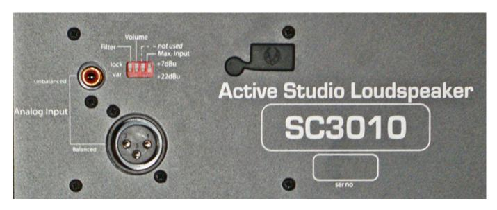
In addition to the input sockets, there are three small DIP switches on the rear of the loudspeaker for selecting the input level and for fixing the current setting of the filters and the input gain too.
