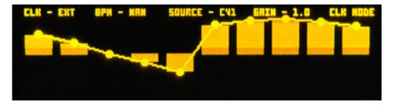
The clock modulation menu is also interesting. Here, you can set a clock source (internal/external), the speed in BPM of the internal clock, the modulation input source (CV1 or all), and a degree of modulation. With an incoming or internal clock pulse, the input value is stored as a sample & hold and assigned to the current filter. With each clock pulse, the corresponding filter number will increase.
