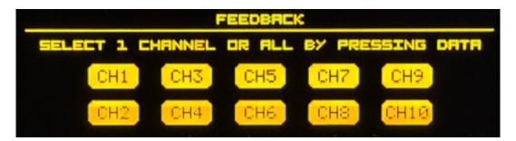
It is interesting to note that you can determine which filters are used for resonance feedback. This can be set globally via the feedback submenu, either all, none or one of the ten filter bands.
