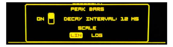
By default, however, it is set to LIN, which means linear; therefore, the display only takes place in a small area on the left. Thus, it is advisable to switch to logarithmic (LOG) if necessary.
