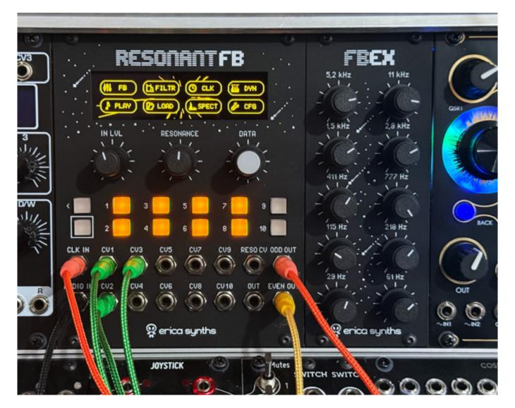
We had a module with firmware 1.2 that we updated to the firmware version 1.3. The update is done by an audio file that is provided on the Erica Synths website. This works best if you play the audio file on a laptop or PC and connect the audio output of the PC directly to the IN socket of the filter module because if you route
