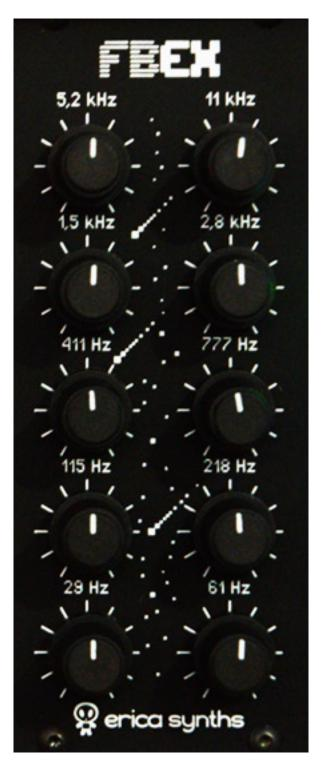
The expander is self-explanatory. The target frequencies of the bands are displayed above the controllers. The ten potentiometers are used to set the gains of the ten bands. As mentioned earlier, there are two operating modes: Offset, where the values are added to those of the filter module, or Attenuate, where the expander settings act as attenuators.
