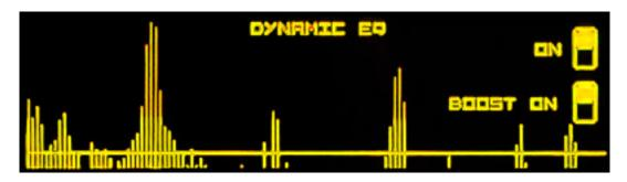
There is also a dynamic equalizer mode, where you can reduce or amplify frequency components depending on a threshold set by the user. The mode can be completely deactivated, and with BOOST ON, you amplify the components that are below the threshold. To see the amplified frequency components, we have set the threshold particularly low for the illustration.
