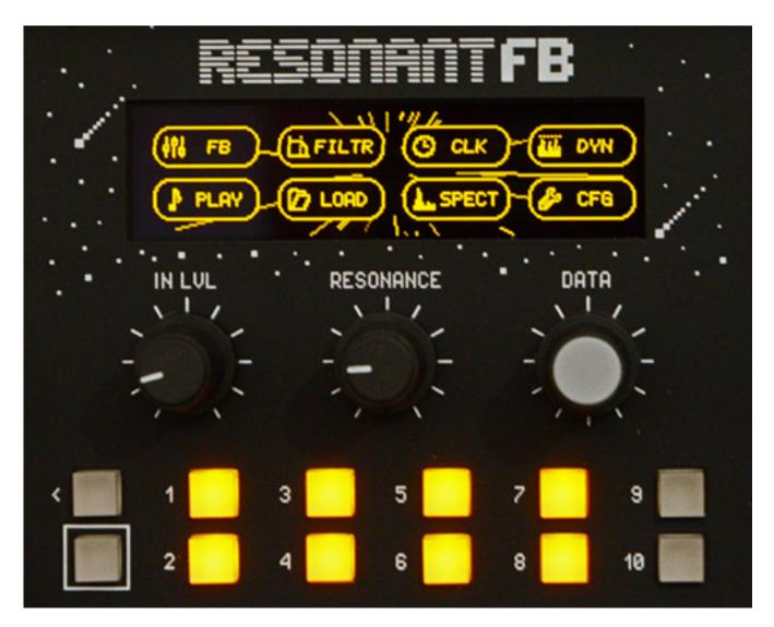
This module is operated via twelve buttons with LED indicators, a controller for adjusting the input level and filter resonance of all bands, as well as a push/turn control for menu selection and parameter entry. A monochrome OLED display measuring 70 x 18mm is included.
