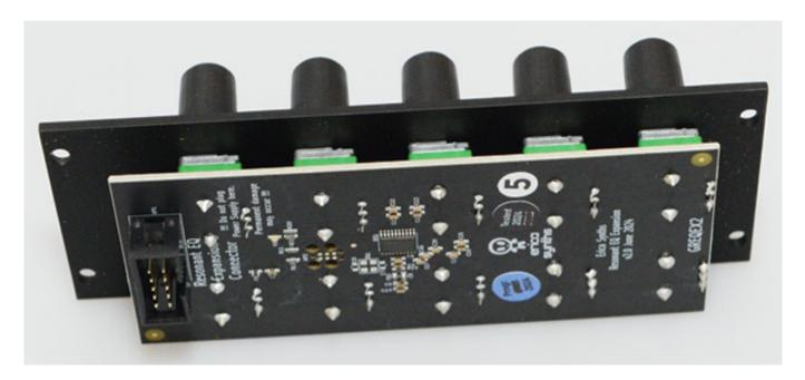
The expander FBEX has a width of 10TE. The mounting depth is only 30mm with the plug. The expander is only connected to the filter module, where it draws its power supply from the filter module. The operating current increases only slightly with the expander module; therefore, the total current with the filter module was on average 118mA and 131mA at peak times in our tests.
