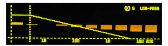
The filters can also be combined to simulate different filter characteristics such as low-pass, band-pass, band-stop and high-pass filters. The pressure/rotary encoder is used to set the cutoff frequency and the shift key can be used to access the filter type setting.
