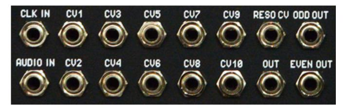
The module has a signal input designed for an audio signal level of 10 volts peak to peak maximum. Internally, there are two filter groups: the odd-numbered (ODD) bands, i.e., 1, 3, 5, 7, and 9, and the even-numbered (EVEN) bands, 2, 4, 6, 8, and 10. These groups are individually routed to 3.5mm jacks and also to a mono sum signal (OUT). The gain can be controlled individually for each band, and the resonance for all filters together. There is also a clock input, which we will discuss later.
