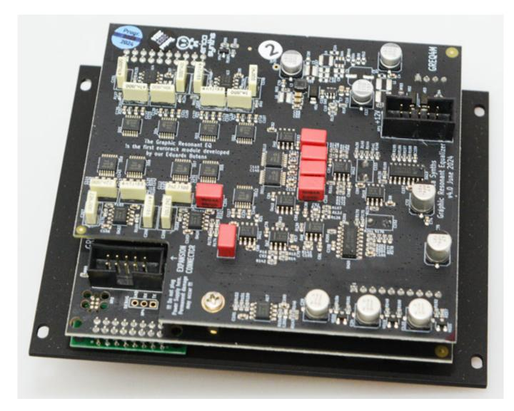
Resonant FB is a 20 HP wide Eurorack module with ten fixed frequency bands: 29, 61, 115, 218, 411, 777Hz, as well as 1.5, 2.8, 5.2, and 11kHz, i.e., approximately one octave apart. The mounting depth with the plug inserted is 43mm. The current consumption of our test module was, on average, 112mA, and at peak times 125mA. The module has two pin strip connectors: one for the power supply and one for the connecting expander.
