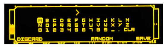
You can use the LOAD menu to reload presets and press the Shift key to access a submenu where you can then rename, move, or delete presets. Up to 128 presets can be stored.
