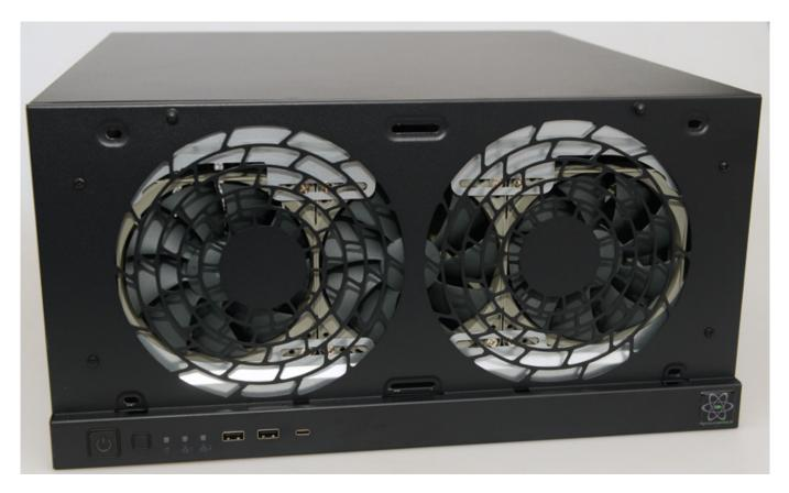
The front grille can be removed to reveal the three 120mm REDUX fans at the front. Another fan can be located at the rear of the housing.
