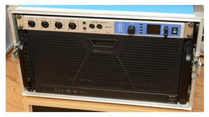
Let us start with the housing. The 19-inch rack brackets on the side are slightly shorter and do not cover the entire 5 U high area. In our rack, it was not possible to use the holes above and below the handle, but this was not a problem, as there are eleven mounting holes on each of the brackets. In contrast to the previous computer, we used a support guide because the weight could be placed in the rack without a support guide for assistance.
