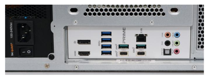
The motherboard's connections also offer a 2.5 GBit/s Ethernet port, as well as six USB-A ports (USB 3.2 Gen 1 and labeled blue with 5 or green with 10 MBit/s) at different speeds and two USB-C ports (USB 3.2 Gen 1 with 10 or 20 MBit/s). A total of 13 USB ports at the back of the entire computer.
