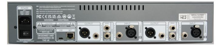
The equipment is completed by XLR in/outs, stereo jacks for the insert path, and an internal power supply unit with a switch and an additional on/off button.
