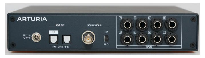
Now let's take a look at the back panel. This is basically the same for both X8 IN and X8 OUT devices, except that inputs or outputs are available. The power connector can be locked. The power supply can be operated in the voltage range from 100 to 240 volts with a mains frequency of 50 or 60 Hz.
