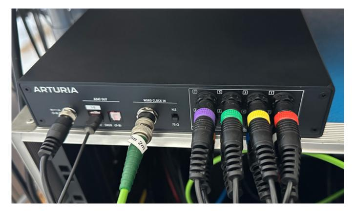
We used the X8 IN to provide an RME MADIface UFX+ with eight additional analog inputs. We tested both master and slave operation. Everything worked perfectly right away. Another tip: many interfaces, like the RME UFX+, have a pair of BNC connectors that can be used either for MADI or for word clock. When operating with the X8 IN, the BNC connector for the output must therefore be switched from MADI to word clock. This should not be forgotten, otherwise the X8 IN will not receive any word clock.
