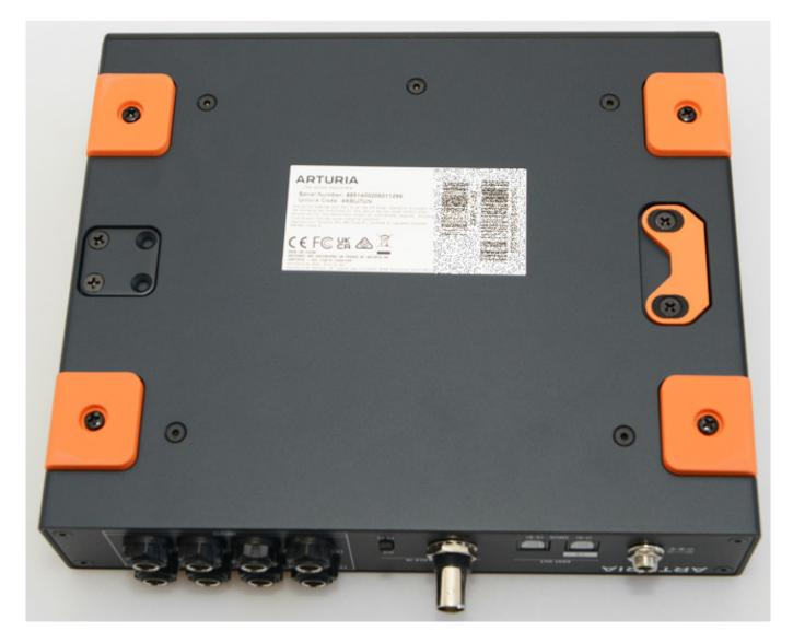
Mounting brackets for installation in a 19" rack are also included. A rack bracket and a connecting plate, along with four screws, are attached to the underside of the unit. The brackets and connecting plate can be unscrewed from the rear. This allows two AudioFuse X8 interfaces, each with a half-rack width, to be joined together to form a single 19" unit and mounted in the rack.
