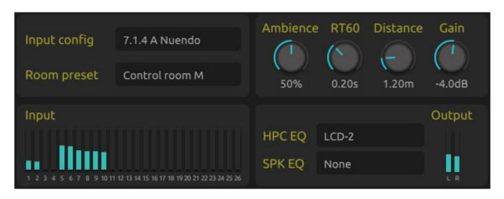
When you switch to another tab, the upper part of the dialog is changed accordingly. The lower area, which contains the input configuration, the preset of the room simulation (APL Listening Room, Control Room small, medium, large, Dubbing Stage, Home Cinema Living Room) and the room simulation parameters, as well as a headphone EQ compensation and an additional loudspeaker EQ curve, is always identical and always available.
