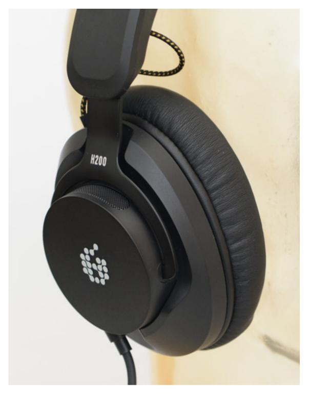
The headphones have circumaural earcups that are acoustically closed. The dynamic driver used has a diameter of 40 mm and an impedance of 32 ohms – so it is relatively low-impedance, like most modern headphones. The sensitivity is 97.5 dB SPL at 1 mW and 1 kHz. The maximum sound pressure is specified by the manufacturer as 112.5 dB SPL (@ 1 kHz, 0.04 % THD). The maximum input power is
