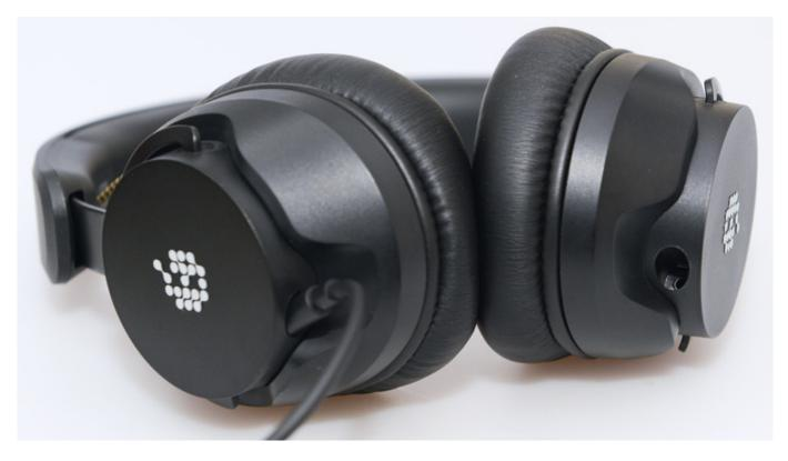
The weight of the headphones is about 250 grams without the cable, and the housing is made of 85 percent recycled ABS plastic. A 2.5-mm jack socket is provided on both sides of the headphones for connecting the headphone cable. The cable can therefore be plugged in on the left or right (see figure above) and is mechanically locked to prevent accidental unplugging.
