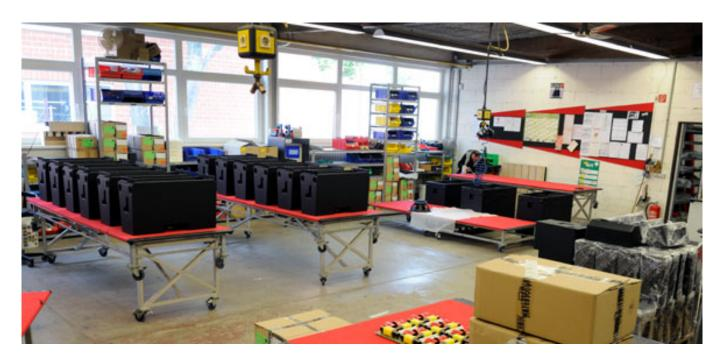
Kling & Freitag is producing speakers for over 20 years and the products are designed and produced directly in Hannover. The drivers are produced by subcontractors according to the special requirements for Kling & Freitag and then mounted in Hannover.
