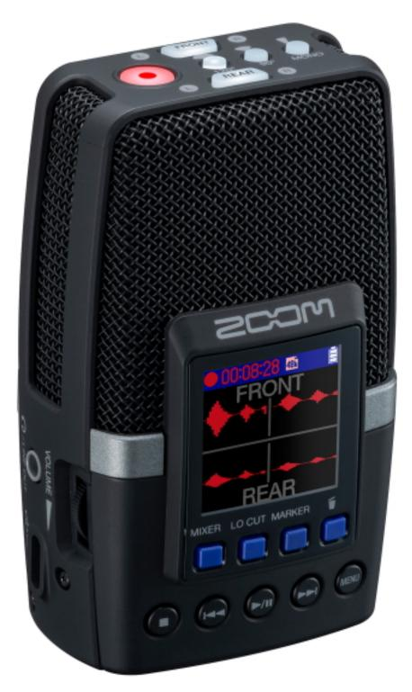
The Zoom H2essential Multi-Mic Handy Recorder is the only Handy Recorder with three internal microphones. With the ability to select different mic patterns, it gives creators more options than ever before. With two cardioid mics facing front and rear and a bi-directional mic facing side to side, the H2essential allows you to choose the perfect pick-up pattern for every recording. Monday, 23 September 2024 17:50
