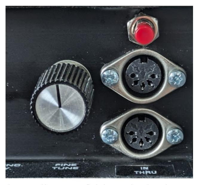
The Kenton Multimoog MIDI Retrofit Kit gives you enhanced control over your Multimoog using MIDI, allowing you to control it from your DAW, sequencer or other controller. You can control notes, modulation, pitchbend and the Multimoog's LFO and filter cut-off. In addition, the MIDI Retrofit Kit gives you sustain and slide/portamento. See below for a full list of features.
