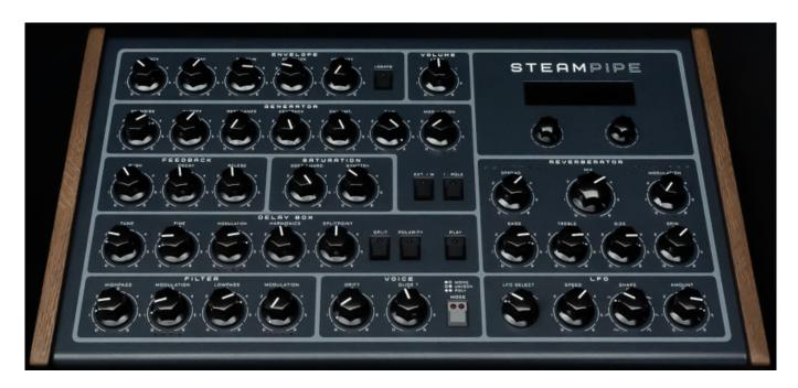
No oscillators, 8 voice polyphony. The Steampipe is a true physical modelling synthesizer developed in close collaboration with Dutch company 112.dB. The Steampipe has no conventional oscillators. Instead, it mimics the way sound is created in wind instruments and it is fine-tuned to create a wide range of sounds -everything from wind instruments to strings, pipe organs, crazy effects and beyond. The Steampipe has three major sections – STEAM, PIPE and REVERBERATOR.
