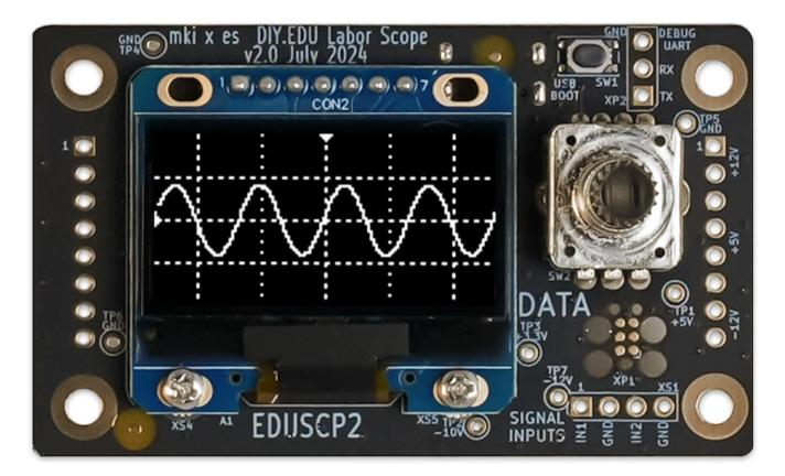
This EDU DIY Labor add-on, featuring the oscilloscope, the voltmeter, the spectrometer and the tuner, turns the, Labor into self-contained electronics development and experimentation station.
