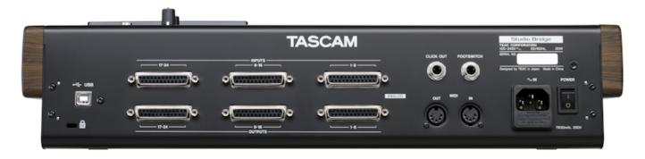
As a USB MIDI interface, the Studio Bridge makes it easy to synchronise with MIDI instruments and devices such as drum machines and sequencers. It also features dual footswitch control for customisable functions and a Mac and Windows control panel, including a meter bridge for visually monitoring signals and adjusting parameters.
