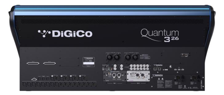
The Quantum326 may also be upgraded with DiGiCo's optional Pulse software update, increasing the console's number of standard input channels to 156 (from 128), busses to 72 (from 64), Mustard Processors to 48 (from 36), and Nodal Processors to 72 (from 64). Another perk of the recent Pulse upgrade is the addition of Mix Minus functionality.
