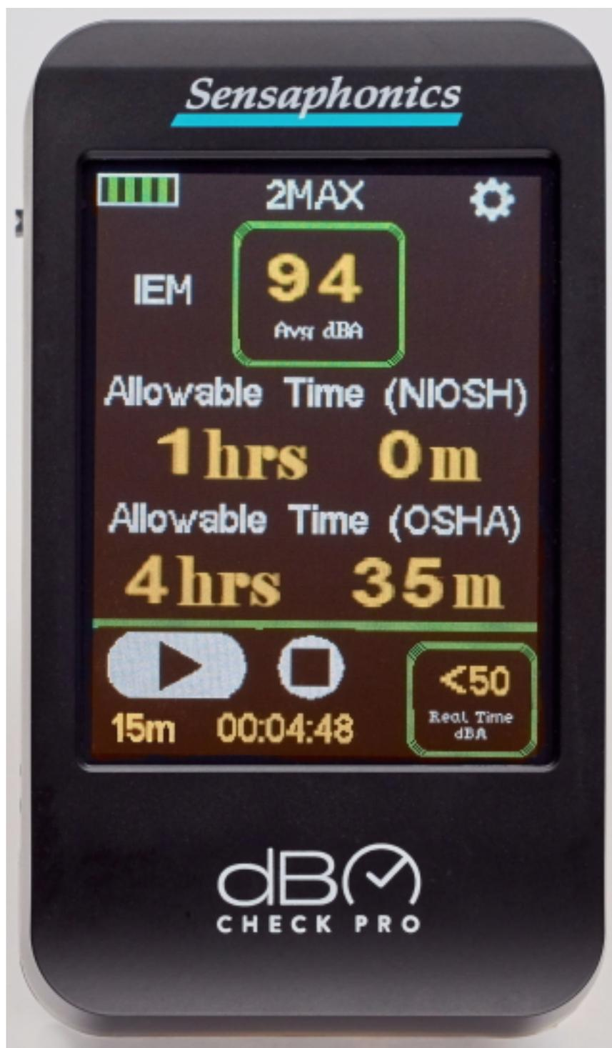
Sensaphonics announces the appointment of ASI Audio, manufacturer of the innovative 3DME in-ear monitoring system, as the exclusive global distributor for its Sensaphonics dB Check Pro, to dealers, distributors, reps and production companies. The dB Check Pro is an in-line, real-time sound level analyzer that shows in-ear SPL and safe exposure times for over 140 professional IEMs and
