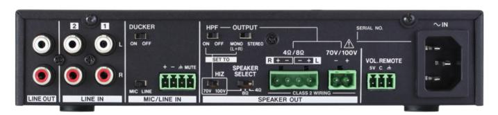
Audio sources can be connected to a Mic/Line input with switchable connectors on the front and rear (the latter supporting paging), a stereo RCA line input and wirelessly via Bluetooth. A Ducker function is available for the mic. Hence, for environments where background music is playing, the system can automatically lower the volume of the music when an announcement is made. With the built-in
