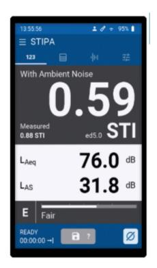
The XL3 Acoustic Analyzer now supports speech intelligibility measurements according to IEC60268-16. Together with the TalkBox (acoustic) and MR-PRO (electrical) signal sources, the XL3 is the ideal tool for efficient and reliable STIPA measurement tasks. The measured values can be conveniently visualized in a report.
