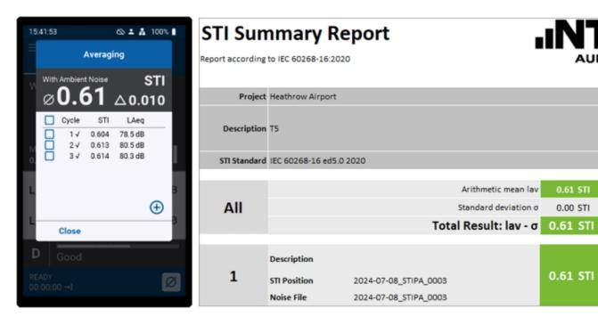
The averaging of multiple measurements at one point is supported by a dedicated screen. Here the user retains the collected information about the individual measurements and the deviations between them. Invalid measurements can be disregarded immediately. With the STIPA Reporting Tool, which is available free of charge, the measurements at several positions can be conveniently summarized in a measurement report.
