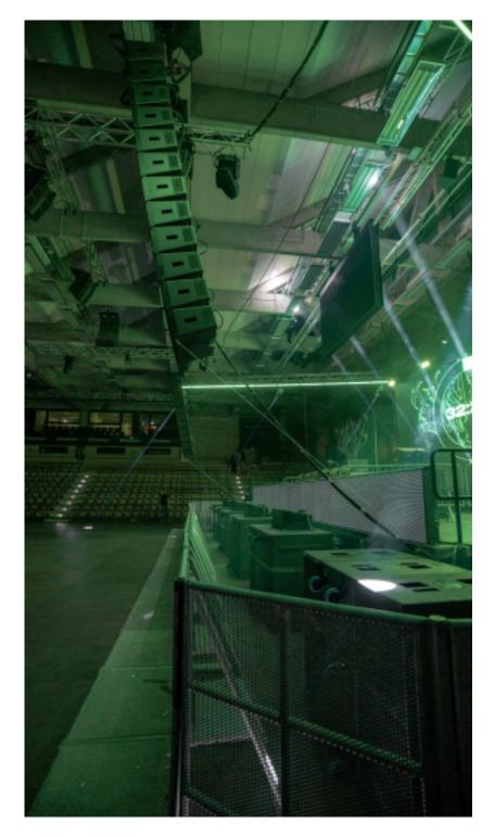
To achieve this Jürgen Schuster deployed 24 Martin Audio WPC as the main system (12 boxes a side), with eight WPS as front- and sidefill. The all-important sub frequencies were pumped out through six towers of three SX218, designed in
