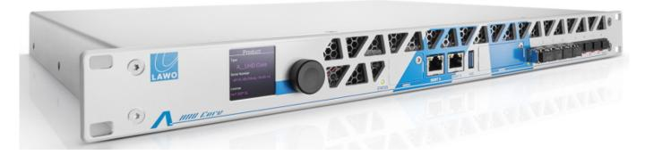
Powering both members of the mc<sup>2</sup> family is the software-defined A\_UHD Core Audio Engine with intuitive HOME functionality. Up to 1,024 mc<sup>2</sup>-quality DSP channels can be shared between multiple consoles based on a flexible licensing system.
