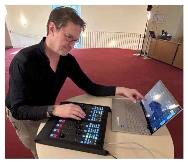
As part of its ongoing advancement of audio infrastructure, Duesseldorf Opera House has chosen to add a Lawo crystal mixing console to its setup. This new console is used wirelessly, primarily to remotely control the larger Lawo mc<sup>2</sup>56 console in the sound control room, allowing flexible, location-independent sound adjustments in the auditorium and other areas, such as the foyer, for smaller events.
